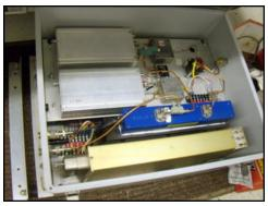
The feed is being prepared and it has a waveguide transition to a Chaparral feed to be mounted once the dish is out of the garage. The RF amplifier and power supply are contained in a large weather-proof box with both 5GHz and 10GHz amplifiers. These were obtained from N3FTI when he downsized his rover station. As we understand, the TWT is capable of at least 40W output.
